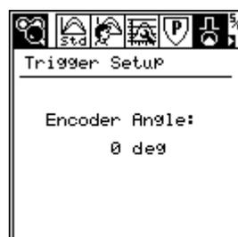
At the Trigger Set-up mode, the triggering edge of the Encoder is automatically detected. Auto-detection of the triggering edge is available for both the Servo and Disc triggering modes.
