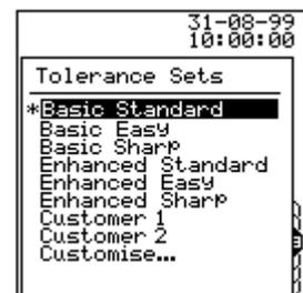
To make changes to the tolerance for the current production, select "Customise..." using the jog shuttle
