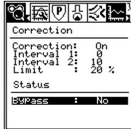
Temporary de-activation of the monitoring function of the Crimp Quality Monitor can be achieved by setting the Crimp Quality Monitor to **Bypass** mode.
