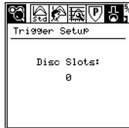
To perform a trigger set-up for the Disc, make a crimp at the selected press, the number of disc slots will be displayed. The ideal number of disc slots obtained should be 110 or 115, to enable correct capturing of the force signals. If the desired disc slots not obtained, please consult SLE Engineers for advice.
