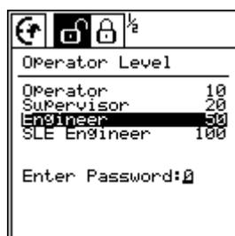
Then, key in the access Password required for the selected Operator Level and press enter
