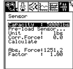
Due to the pivot construction of the baseplate where the piezo force sensor is installed, the force measured by the sensor may only be a fraction of the actual force.
