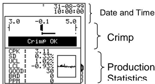
If 2-CH View is selected, it will be able to display the crimp details and the production statistics of both the crimp presses.
