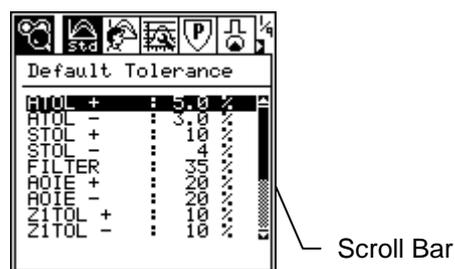
The Default Tolerance settings provide a default set of working tolerances that is used for quality assurance purposes in the production after a Learn is performed.
