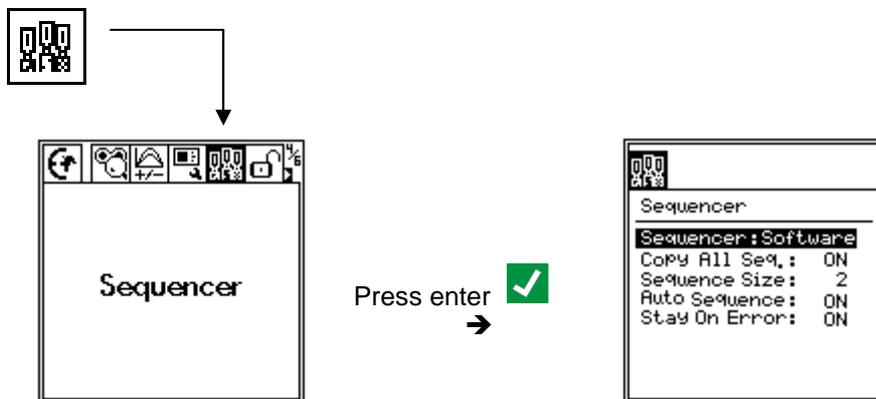
While highlighting the desired option as shown above, changes can be made by pressing enter
