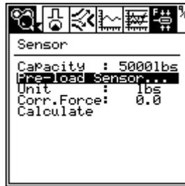
Ensure that the force sensor is free of stress or load. Unscrew any screws that might have directly or indirectly exerted any force or load on the force sensor. Then, press enter
