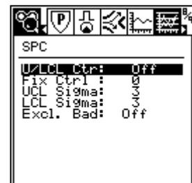
If **U/LCL Ctrl (UCL & LCL Control)** option is selected, the area evaluation of the crimping force will be **based on** the tolerance given by the UCL and LCL of the statistical process computed.
