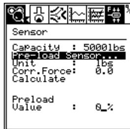
At this instant, the Crimp Quality Monitor records the current stress condition as the reference stress or load and assign a zero value to it. Any additional tension or extension force will then be recorded relatively and the relative percentage will be updated and shown on the display as the pre-load value for the sensor.
