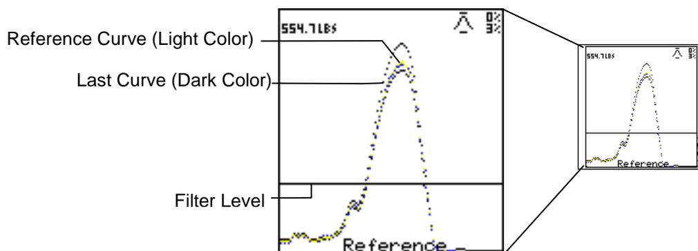
The normal operation mask is restored after the Reference curve is displayed for three seconds.
