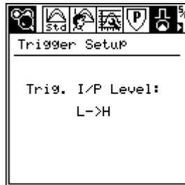
Here, the **Trig. I/P Level (Triggering Input Level)** of Proximity is detected. Once the triggering input level is obtained, the trigger set-up is completed.
