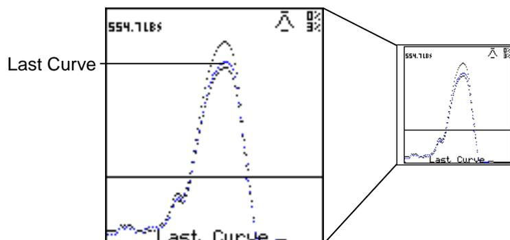
To toggle between the Last Curve and the Reference Curve view, rotate the jog shuttle
