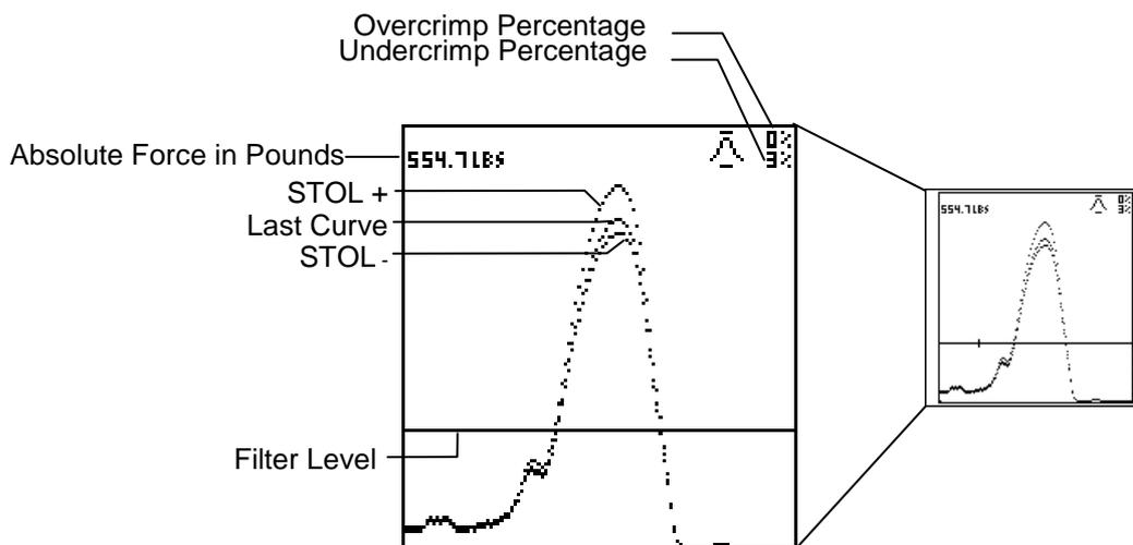
During the production process, the undercrimp and overcrimp percentages of each crimp are evaluated based on the Crimp Shape analysis method and displayed at the top right hand corner of the curve.
