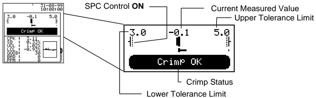
If **Fix Ctrl (SPC Control)** option is selected, the UCL and LCL values used for area evaluation will be kept constant after the number of crimps specified in the **Fix Ctrl** field occurs.
