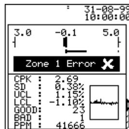
If the Crimp Quality Monitor system is being programmed to stop at every fault detected, the STOP output relay will be opened to stop the crimping press or the automatic cutting machine. To run the production again, the error occurred in the press needs to be reset.
