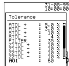
The maximum values of the tolerance parameters are limited by the User's Limits (see *Programming Guide ~ Parameter Setup ~ User's Limits*).
